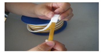
• By removing the protective strip, without adopting the correct procedure as described above, the adhesive strip shall remove from the expanded PTFE tape, thus causing difficulty during installation.
